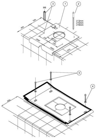
Figure 5 - Fixation of the OSB11
