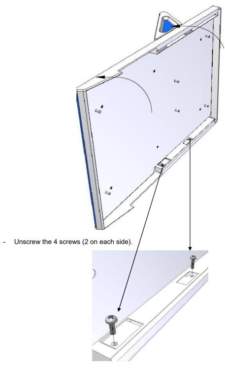
Figure 10 - Dismantling of the footrest
