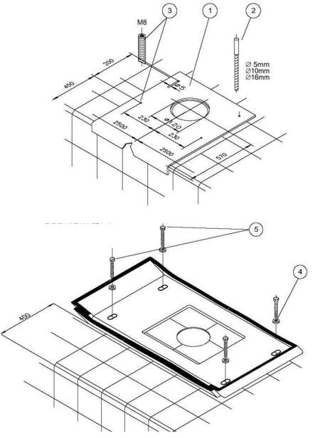
Figure 3 - Fixation of the starting block
