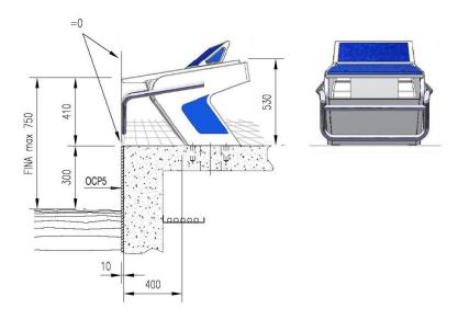
Figure 4 - Positioning of the OSB11
